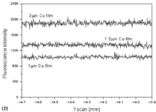
**Fig. 3** Fluorescence measurement of un-shocked copper thin films with X-ray energy at 9.1 KeV (a) Fluorescence spectra of the copper thin films; and (b) Fluorescence intensity distribution across the film surface, step size 2 microns
