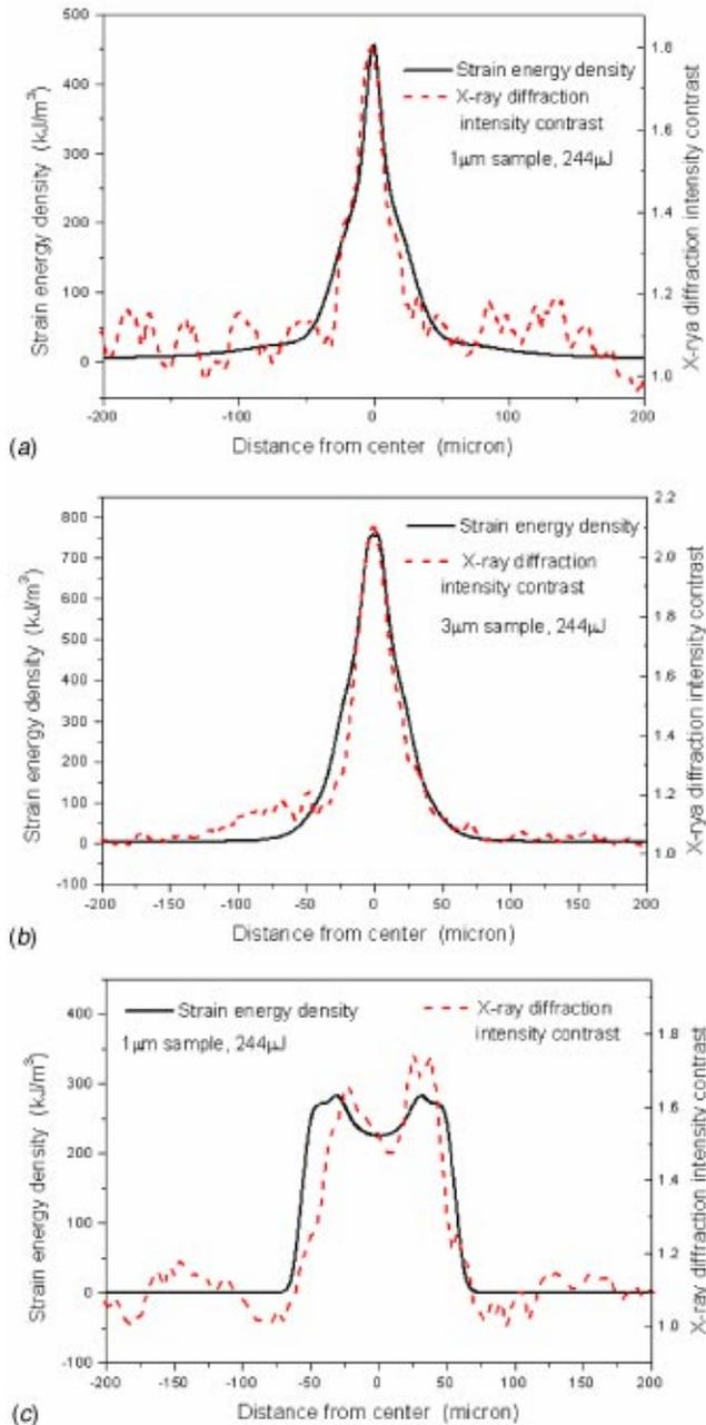
**Fig. 7 Comparison of strain energy density (solid line) and X-ray diffraction intensity contrast (dashed line) (a) 1  $\mu\text{m}$  sample, 244  $\mu\text{J}$ , single line; (b) 3  $\mu\text{m}$  sample, 244  $\mu\text{J}$ , single line; and (c) 1  $\mu\text{m}$  sample, 244  $\mu\text{J}$ , 7 lines**
