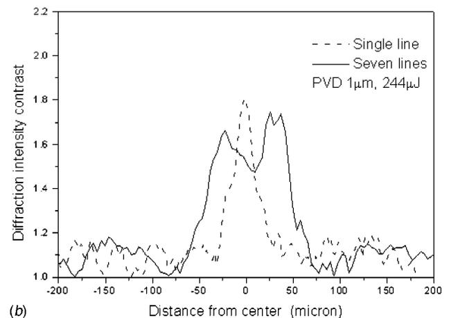
**Fig. 4** Si (004) diffraction intensity contrast across the shocked region measured in 2-micron step size. (a) pulse energy of 244  $\mu\text{J}$  and 209  $\mu\text{J}$ , 3  $\mu\text{m}$  sample, single line shocking; and (b) Comparison of single line and 7 line shocking results, pulse energy of 244  $\mu\text{J}$ , 1  $\mu\text{m}$  sample. The diffraction intensity is normalized to the average background diffraction intensity (14000 counts).
