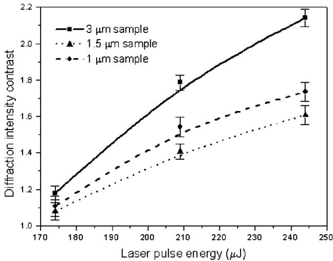
**Fig. 5** Variation of diffraction intensity contrast with laser pulse energy and film thickness. Each data point represents the average of three measurements, standard error is used to plot the error bars, and smooth lines are fitted through these data points. The diffraction intensity is normalized to the background diffraction intensity counts
