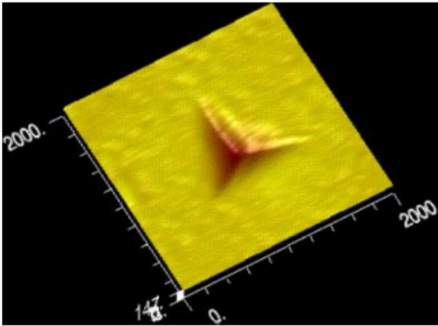
**Fig. 8** 3D image of the indentation on the un-shock 1  $\mu\text{m}$  copper thin film on silicon substrate. Berkovich diamond nanoindenter leaves a triangular dent in the sample. The unit in the image is nm. The full scale in the depth direction is 147 nm. The maximum loading is 1000  $\mu\text{N}$ .
