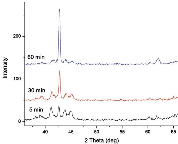
**Fig. 8 XRD spectra for films annealed at 560°C for various times. Note growth of austenitic peaks (42.8 deg and 61.8 deg) and decay of martensitic peaks with increasing annealing time. Spectra shifted for clarity.**
