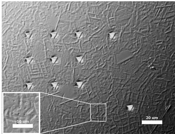
**Fig. 11** Optical micrograph of residual impressions from 1  $\mu\text{m}$  and 100 nm (inset) deep indentations on annealed NiTi film before heating. Film annealed at 460  $^{\circ}\text{C}$  for 5 min.
