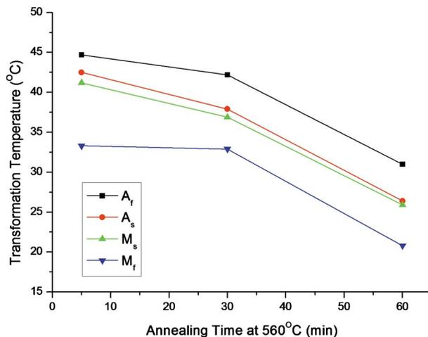
**Fig. 6 Transformation temperatures versus annealing time for films annealed at 560°C. Measured through in situ temperature dependent optical microscopy. Transformation temperatures could not be measured for samples annealed at 760°C.**
