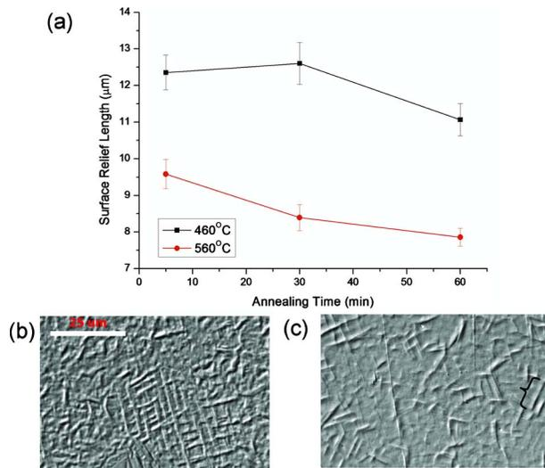
**Fig. 3** (a) Length of martensitic surface relief as a function of annealing parameters. Error bars denote standard error. Optical micrographs of samples annealed at (b) 460°C for 5 min and (c) 560°C for 60 min (surface relief length denoted by bracket).
