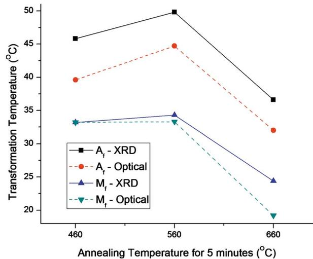
**Fig. 10 Transformation temperatures of samples annealed for 5 min as a function of annealing temperature. Comparison between XRD and optical methods. Austenitic start ( $A_s$ ) and martensitic start ( $M_s$ ) omitted for clarity. Transformation temperatures could not be measured for samples annealed at 760°C.**
