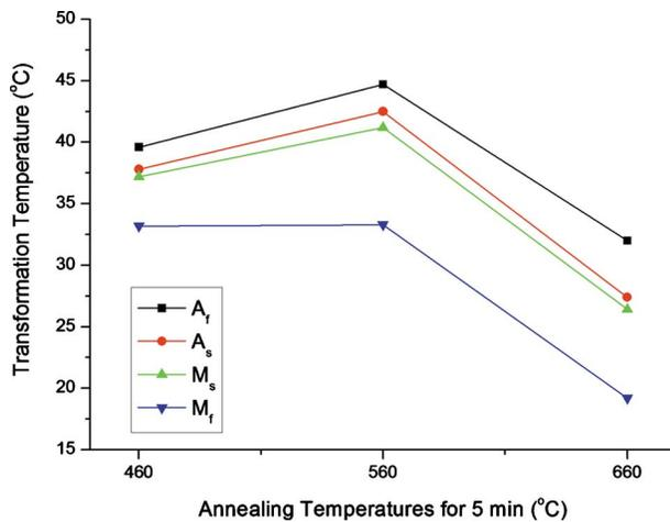
**Fig. 5 Transformation temperatures versus annealing temperature for films annealed for 5 min. Measured through in situ temperature dependent optical microscopy. Transformation temperatures could not be measured for samples annealed at 760°C.**
