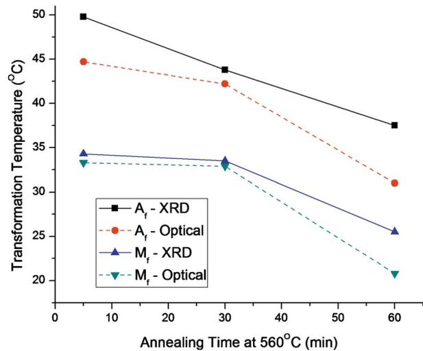
**Fig. 9 Transformation temperatures of samples annealed at 560°C as a function of time. Comparison between XRD and optical methods. Austenitic start ( $A_s$ ) and martensitic start ( $M_s$ ) omitted for clarity.**
