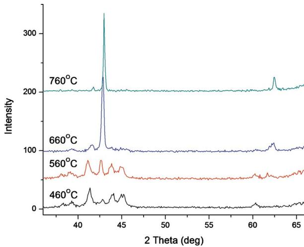
**Fig. 7 XRD spectra for films annealed for 5 min at various temperatures. Note growth of austenitic peaks (42.8°C and 61.8°C) and decay of martensitic peaks with increasing annealing temperature. Spectra shifted for clarity.**
