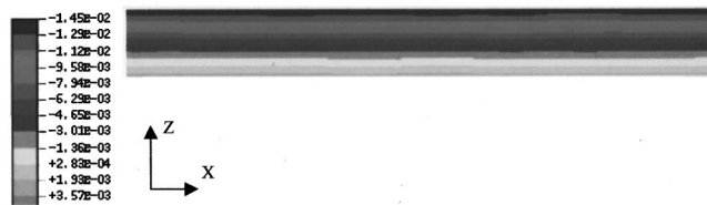
(a) Portion (8 mm long) of the symmetric plane (0.89 mm thick and 40 mm long) (Power=843W, Velocity=90mm/s)
