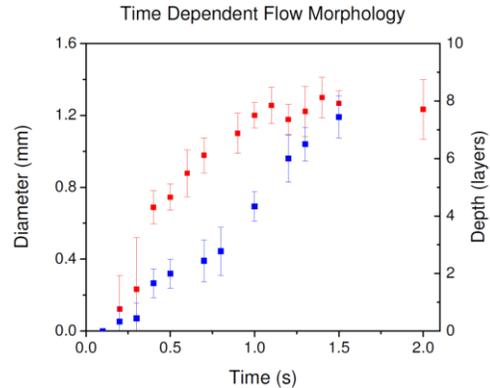
**Figure 3:** Measurements from optical micrographs of the morphological evolution of an in depth joint as a function of time. Note that the diameter of the melt ring reaches a steady state and plateaus while the depth of laser penetration is observed to be approximately linear up to the maximum thickness tested.
