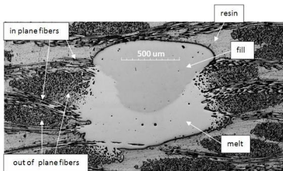
**Figure 7:** Cross section optical micrograph taken of a four layer through thickness joint cross section. Note that the joint is mostly dense with little to no porosity in the through thickness. The Soda Lime fill glass is observable in optical images from the contrasting index of refraction from the E-glass fiber melt.
