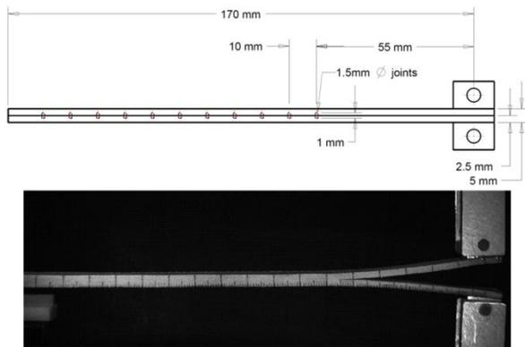
**Figure 9:** Sample schematic of a laser joined DCB specimen and still image of DCB test during displacement controlled loading. Synchronized capturing of high resolution DCB fracture images enables the calculation of fracture energy with high spatial resolution.
