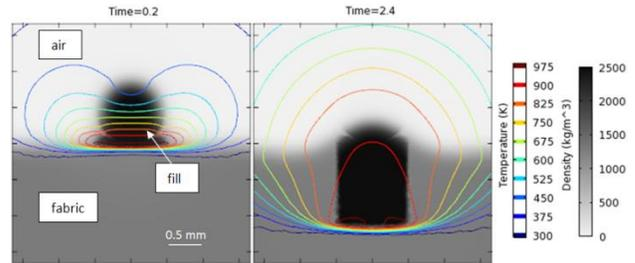
**Figure 8:** Numerical simulation snapshots of fill induced joining showing the time dependent evolution of the melt morphology during laser fusion joining. Void formation in the substrate is observed to be suppressed by the addition of the fill material. The temperature and morphology of the joint is otherwise shown to be unchanged from the non fill simulation.
