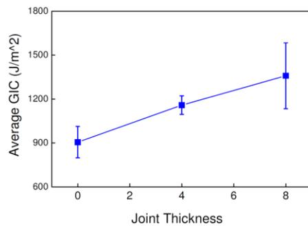
**Figure 11:** Compiled data of the average DCB fracture energy as a function of joint thickness. Note that the average fracture energy follows an approximately linear trend with the joint thickness due to the higher maximum load and peak fracture energies exhibited at the joint locations.
