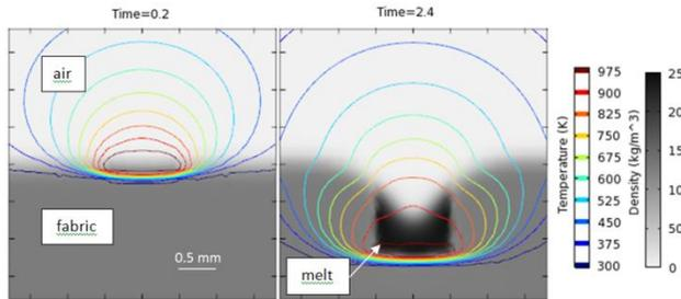
**Figure 4:** Numerical output of the glass densification process without filler material. The substrate is shown to form a void in the center of the laser focus with the maximum temperature at the base of the laser penetration depth.
