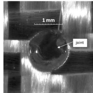
**Figure 6:** Optical micrograph of a through thickness joint with fill. Note that the center of the joint is fully dense glass with little to no porosity, relatively more transparent than the surrounding fabric.
