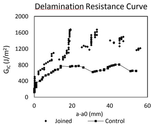
**Figure 10:** Characteristic DCB fracture energy showing significantly higher fracture energy at joint locations corresponding to the discontinuous load profile observed in the load versus crack length output.
