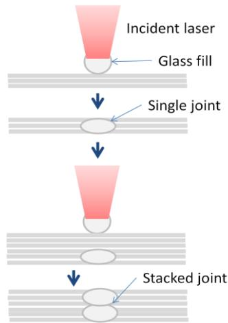
**Figure 1:** Inter laminar joining process schematic showing the layered building process of laser fusion joining. Each joint is aligned with the joint below it to form a continuous stack of joints in the through thickness.
