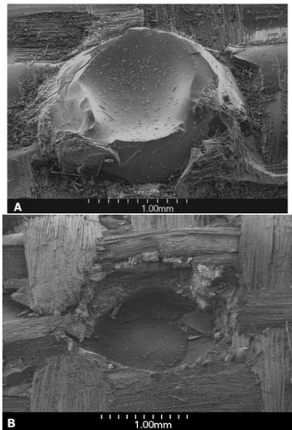
**Figure 12:** SEM images of joint fracture surfaces showing fiber fracture and crack branching behavior due to crack deflection at joints. A positive and negative imprint of the joint remains after the crack has propagated around the joint.
