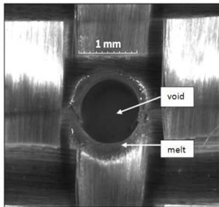
**Figure 2:** Optical micrograph of the surface fiber morphology after laser irradiation of a single layer of plane woven fabric. A dense ring of glass is formed during the heat induced compaction of fibers within the fabric.
