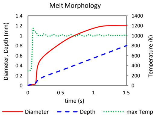
**Figure 5:** Numerical output of the time dependent joint morphology: temperature depth and diameter as a function of time. The melt diameter and depth is shown to follow the same trend as the experiments observed under optical microscopy.
