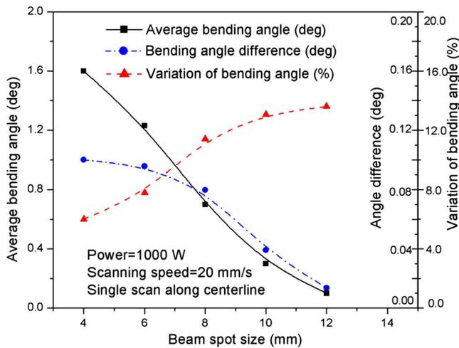
Fig. 11 Bending deformation of varying-thickness coupon under various beam spot sizes (power=1000 W, scanning speed =20 mm/s, single scan along the centerline)
