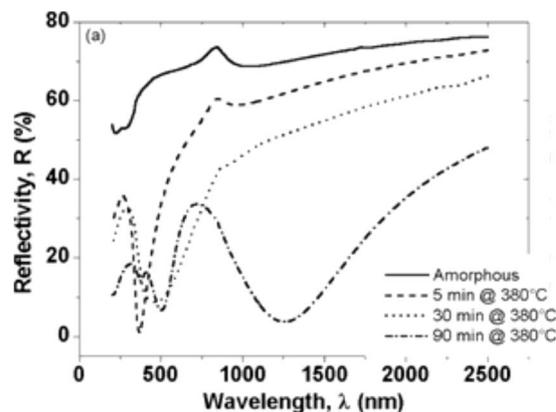
FIG. 4. Reflectivity spectrum for an amorphous and a number of heat treated films. This change in reflectivity, due to oxidation, particularly at  $\lambda = 308$  nm, is consistent with observed enhanced laser-film energy coupling (Ref. 29).
