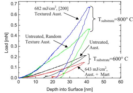
FIG. 12. (Color online) Load responses of laser treated and untreated films for elevated substrate temperatures of  $600^\circ\text{C}$  and  $800^\circ\text{C}$ . Note the increased slope as well as increased depth recovery for the laser treated, [200] textured film treated at  $800^\circ\text{C}$ . The load response of a precrystallized (no laser treatment) film at  $800^\circ\text{C}$  is also included for reference.
