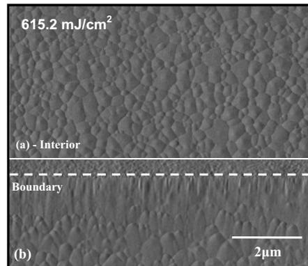
FIG. 14. [(a) and (b)]  $T_{\text{substrate}} = \text{room temperature}$ : representative AFM image from completely melted film. Note the presence of lateral growth, although not well defined or of significant length,  $ED=615.2 \text{ mJ/cm}^2$ .
