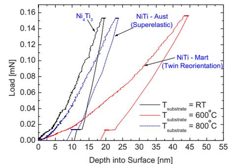
FIG. 10. (Color online) Load curve comparisons between specimens processed at room temperature ( $ED=650 \text{ mJ/cm}^2$ ), 600 °C ( $ED=643 \text{ mJ/cm}^2$ ), and 800 °C ( $ED=682 \text{ mJ/cm}^2$ ). Note that all specimens presented here were laser treated with energy densities above their respective CMTs.
