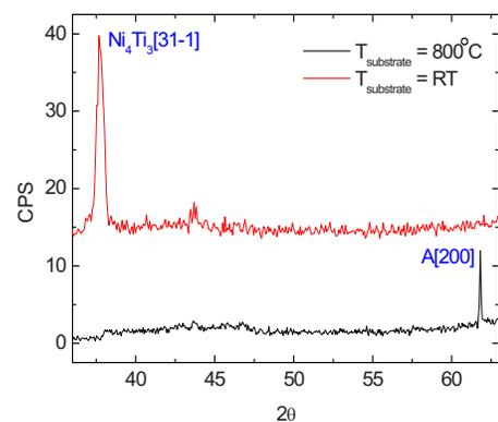
FIG. 8. (Color online) XRD spectra for room temperature and  $800^\circ\text{C}$  substrate temperature. Room temperature processing ( $\text{ED}=650 \text{ mJ/cm}^2$ ) results in metastable phase formation, while an elevated substrate temperature processing ( $\text{ED}=682 \text{ mJ/cm}^2$ ) results in the formation of austenite. Note that both films were laser treated above their respective complete melt thresholds and result in highly textured films implying heterogeneous nucleation.
